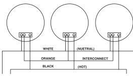
UNSWITCHED 120V AC 60HZ SOURCE TO ADDITIONAL ALARMS MAX. OF 18 INTERCONNECTED
