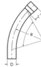
SCH 80 SPECIAL RADIUS ELBOW BELL END 45° 36" RADIUS
