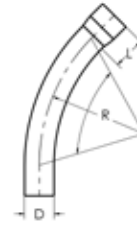
SCH 80 SPECIAL RADIUS ELBOW BELL END 45° 24" RADIUS
