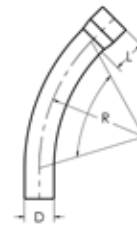
SCH 80 SPECIAL RADIUS ELBOW BELL END 45° 48" RADIUS
