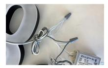
Once all numbers are secured against the mounting plate/surface, gather the grey wire from each number and cut to desired length ensuring wires are long enough to connect together and to power source. Strip grey wire covers ½" then twist the wires together. Join the twisted number wires with the end of the wire marked with +12VDC of the power source and slide the wire cap onto the wires and twist clockwise to secure the wires together.
