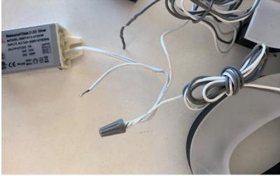
Repeat step 8 for the white wires behind each number – cut and strip each white wire then twist stripped ends together. Join the end of the wire marked with -12VDC of the power source with the joined white wires and slide the wire terminal cap over all of the wires and twist clockwise to secure these wires.
