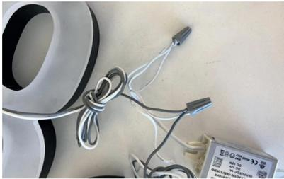
Once all numbers are secured against the mounting plate/surface, gather the grey wire from each number and cut to desired length ensuring wires are long enough to connect together and to power source. Strip grey wire covers  $\frac{1}{2}$ " then twist the wires together. Join the twisted number wires with the end of the wire marked with +12VDC of the power source and slide the wire cap onto the wires and twist clockwise to secure the wires together.
