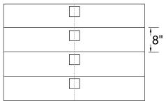
Mount in center of stair as close to the upper tread as possible. For best results use one light per step for steps narrower than 5'.
